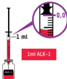
edge of the black plunger ring must sit exactly on the 0,0 ml mark (see diagram). A small air bubble under the plunger will not interfere with the test.
